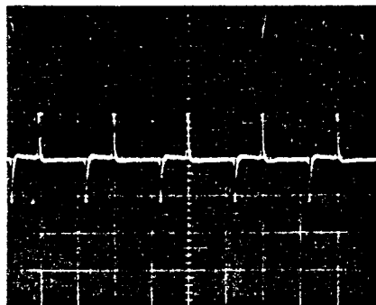
IC704 PIN 6 PB 2V/20msec. div.
